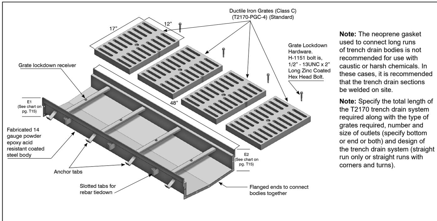
**Note:** The neoprene gasket used to connect long runs of trench drain bodies is not recommended for use with caustic or harsh chemicals. In these cases, it is recommended that the trench drain sections be welded on site.
