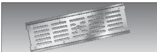
**T1400-PGV-LG-4-3** ductile iron longitudinal slotted grate with Type 304 stainless steel veneer. Horizontal slots for increased intake ability. Illustrated with cast iron frame and Type 304 stainless steel veneer assembly. Must order assembled as illustrated.
