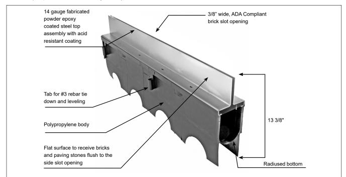
**Note:** Specify the total length of the T1400-SD-BRS slot drain system required along with the number of outlets (specify bottom or end or both) and design of the trench drain system (straight run only or straight runs with corners and turns). MIFAB®'s Engineering team will produce a sign off drawing illustrating the T1400-SD-BRS trench drain system requested for customer sign off and then MIFAB Customer Service quotation.
