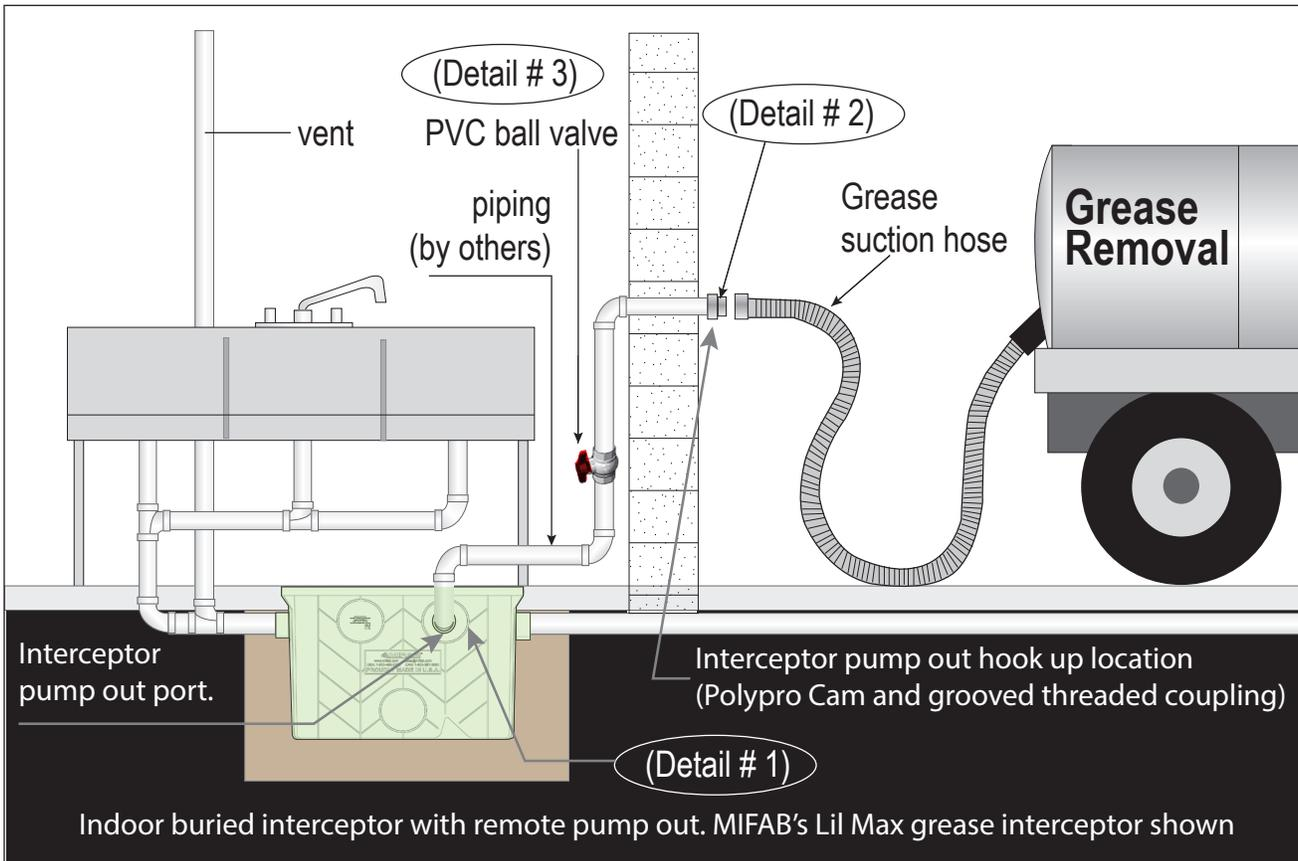
Indoor buried interceptor with remote pump out. MIFAB's Lil Max grease interceptor shown
