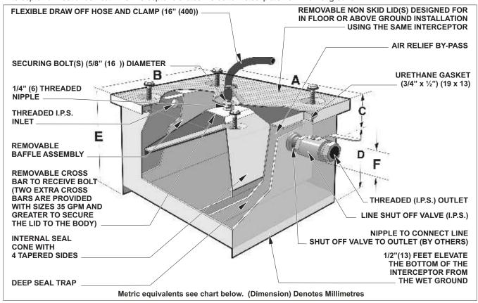
**Note:** The "C" dimension detailed above is from either the middle of the inlet or the outlet to the top the interceptor. The inlet and outlet dimensions are always the same.
