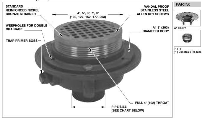
F110-C - FLOOR DRAIN WITH 7" DIA.CAST IRON BODY AND ROUND, ADJUSTABLE NICKEL BRONZE STRAINER -WITH MEMBRANE CLAMP AND TRAP PRIMER TAPPING AND PLUG
