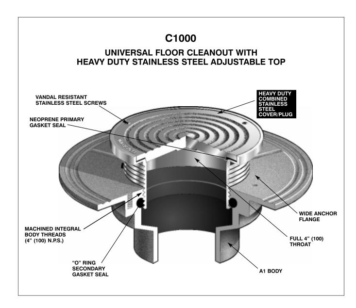
C1000, C1100 SERIES HAVE BEEN TESTED AND CERTIFIED TO THE ANSI/ASME CLEANOUT STANDARD A112.36.2M-1991 AND ARE LISTED WITH I.A.P.M.O.
