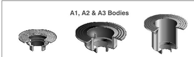
rates. The shallow design of the A1 body allows for installation in slabs of minimum thickness. **Because a membrane clamp is usually not required (the majority of drains and cleanouts are installed slab on grade), MIFAB's A1 body design incorporates an integral female thread (4" N.P.S.M.) to receive adjustable strainers or cleanout tops.**
