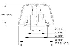
**Note:** Universal body assembly fits over 2", 3" or 4" vertical vent pipe. One size serves all three different outlet sizes. For 6" vertical vent pipe, discard the internal "step" piece and use the three securing screws to assemble the cast iron vent cap to the top of the 6" vertical vent pipe.
