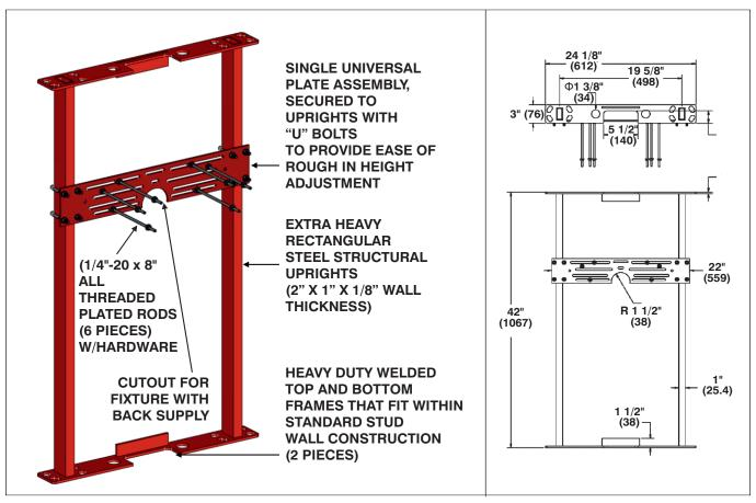
NOTE: Foot supports should be securely anchored to floor with 1/2" bolts and anchors by others
