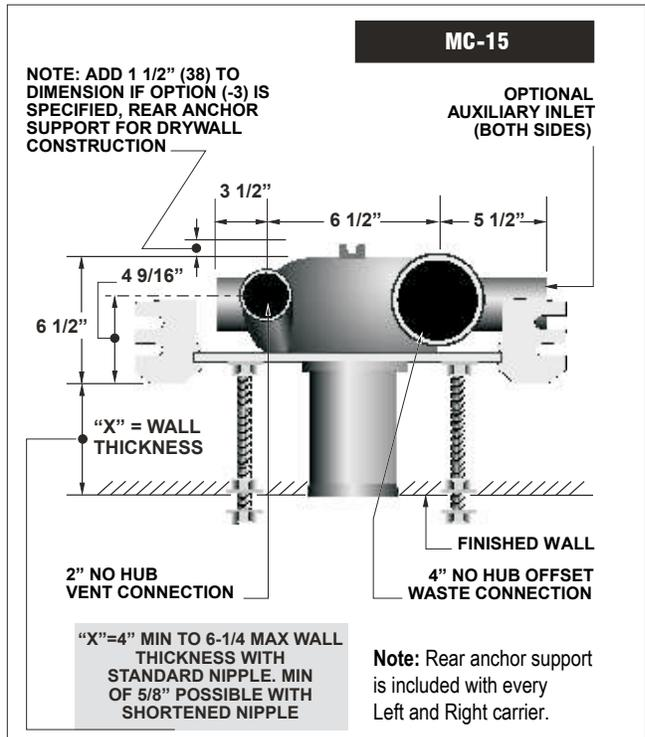
**MC-15 Series Meets ANSI/ASME fixture carrier standard A112.6.1M-97 500Lb. Load Rating**
