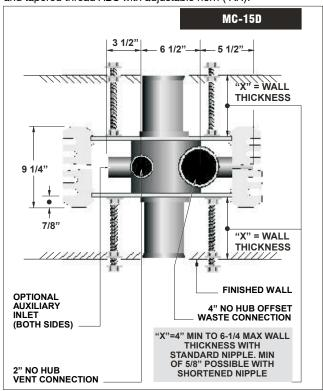
MC-15D Series Meets ANSI/ASME fixture carrier standard A112.6.1M-97 500Lb. Load Rating
