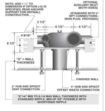
Note: Rear anchor support is included with every Left and Right carrier.
