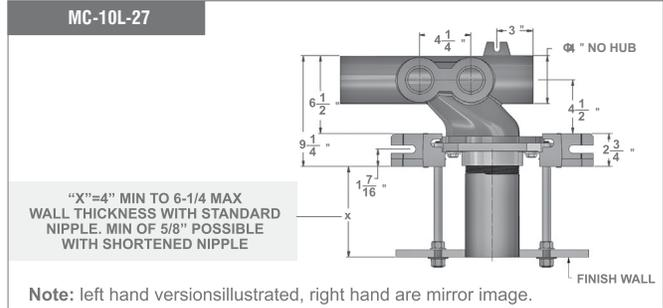
\*MC-10-27 is tested to support a 500 lb. load with the rear anchor support.
