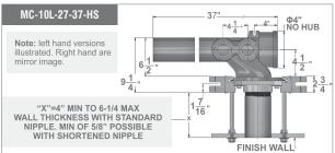
4 1/8" DIMENSION BETWEEN AUXILIARY INLET AND VENT IS IDEAL FOR A STANDARD WYE AND 1/8th BEND CONNECTION
