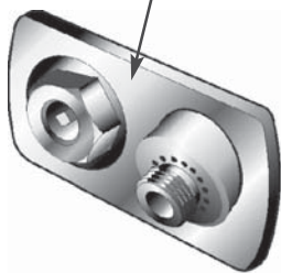
HYDRANT FACEPLATE IN CORRECT HORIZONTAL POSITION
