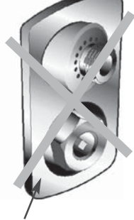
HYDRANT FACEPLATE IN INCORRECT VERTICAL POSITION
