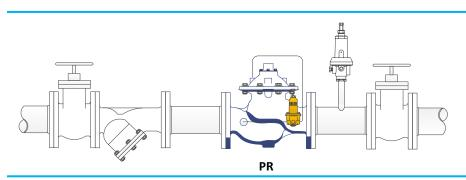
The Model PR reduces high pressure from near zero to the maximum flow rate without the need for an additional Low-Flow Bypass. If the system is subjected to potentially static downstream conditions, a Pressure Relief Valve (½" or larger) is recommended for additional system protection.
