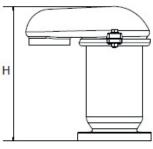
Connections: ISO, ANSI, BS, JIS flanges, BSP, NPT threads (50mm valves only)
