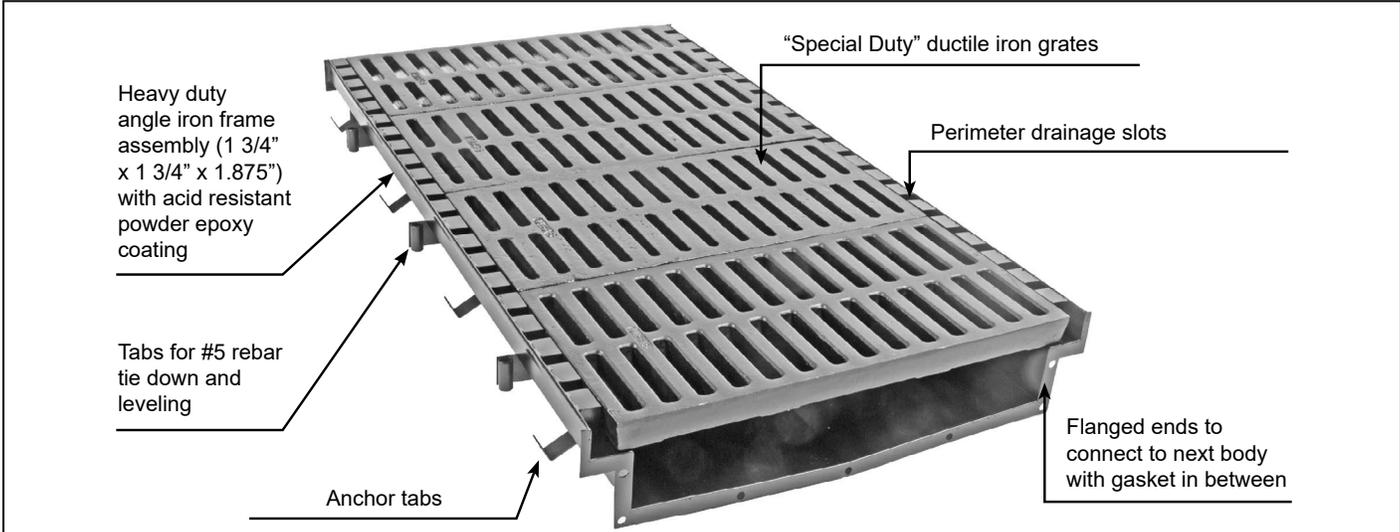
**Note:** Specify the total length of the T2600 trench drain system required along with the type of grates required, number and size of outlets (specify bottom or end or both) and design of the trench drain system (straight run only or straight runs with corners and turns). Each 48" long body section is sloped 1% from one end to the other.
