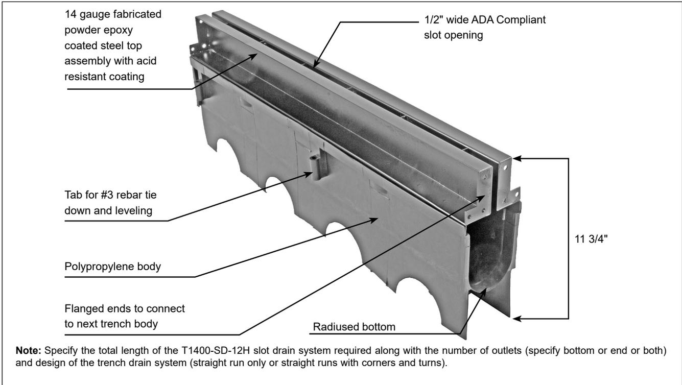
**Note:** Specify the total length of the T1400-SD-12H slot drain system required along with the number of outlets (specify bottom or end or both) and design of the trench drain system (straight run only or straight runs with corners and turns).
