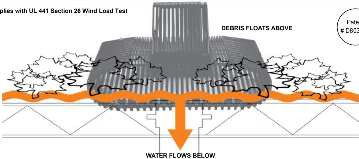
With RoofGuard on duty 24/7, protected roof drains should only require an annual inspection and cleaning to remove accumulated seasonal debris.
