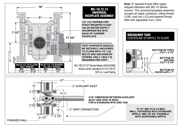
Note: 14 1/2" (368) minimum space required between front of foot supports. 9" (229) minimum in wall space required between back of in wall foot supports.
