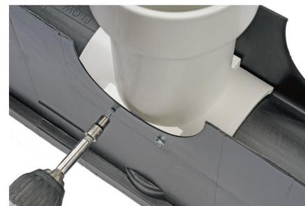
**BOTTOM OUTLET ASSEMBLY:** Once you have positioned the outlet, use 1/2" self-tapping screws. The outlets have bosses that flush out against the channel walls/feet. Tap screws through the outside of the wall into the boss areas on each side of the outlet.
