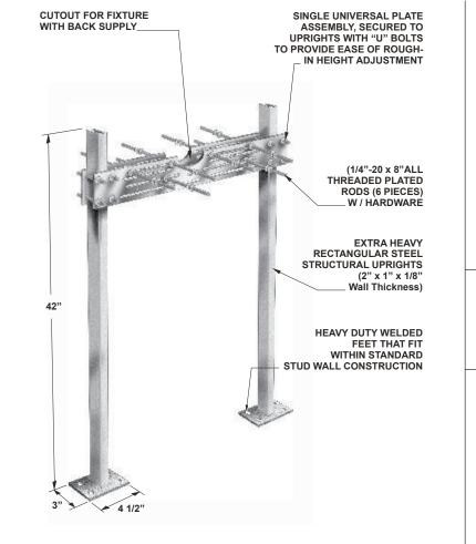
MC-31D Series Meets ANSI/ASME fixture carrier standard A112.6.1M-97
