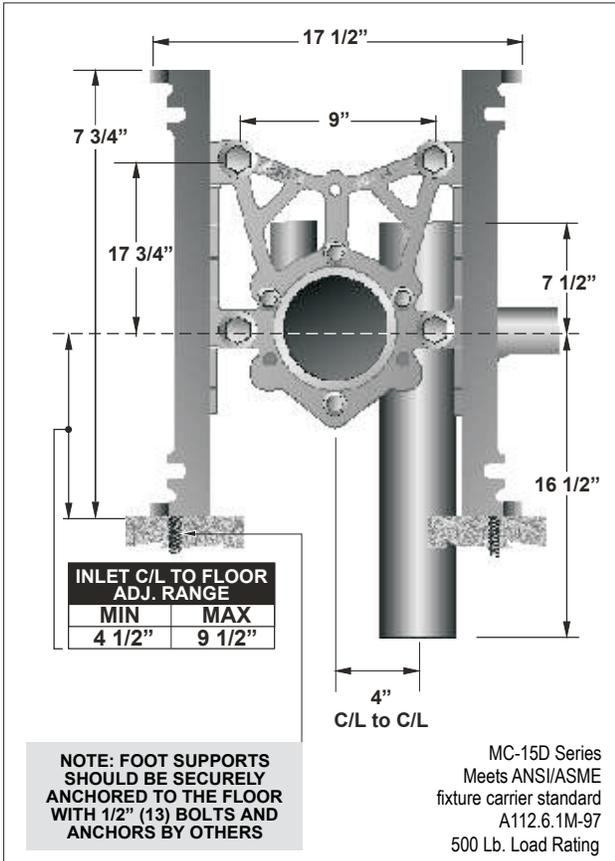
**Note:** 8" tapered thread ABS nipple shipped standard with MC-15D Series carriers. The universal faceplate assembly accepts all nipple variations, rolling thread (-OR), cast iron (-CI) and tapered thread ABS with adjustable horn (-AH).
